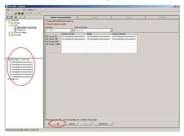
In order to fill the table it is required to click the respective standard measurement, which is listed, with the left mouse button and to drag it into the relevant field of the table. To do this the left mouse button has to be pressed till cursor is above the relevant field (drag and drop). If all fields are filled in by using this procedure the edit mode can be left by pressing the "OK" button.
