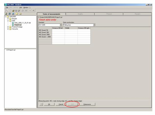
First of all it is required to choose the relevant standard and the type of object on which the project is based from the pull-down menus. A table below the pull-down menus shows the required measurement points for the chosen type of door/gate. The respective measurements from the KMG 2000 L have to be filled into this table.
